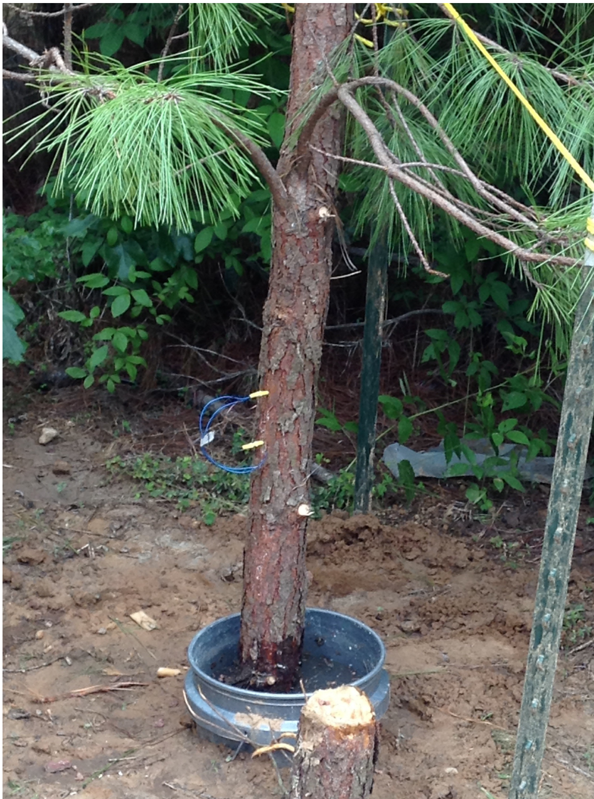
Sap flow and transpiration rate data collection (courtesy of Oklahoma NSF-funded EPSCoR's 2014 Summer Authentic Research Experience for Teachers (ARET))
