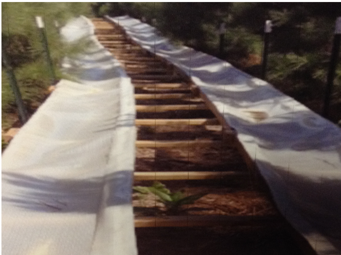
Rainfall excluders on drought plots carry 30% of rainfall off of the plot to simulate drought
