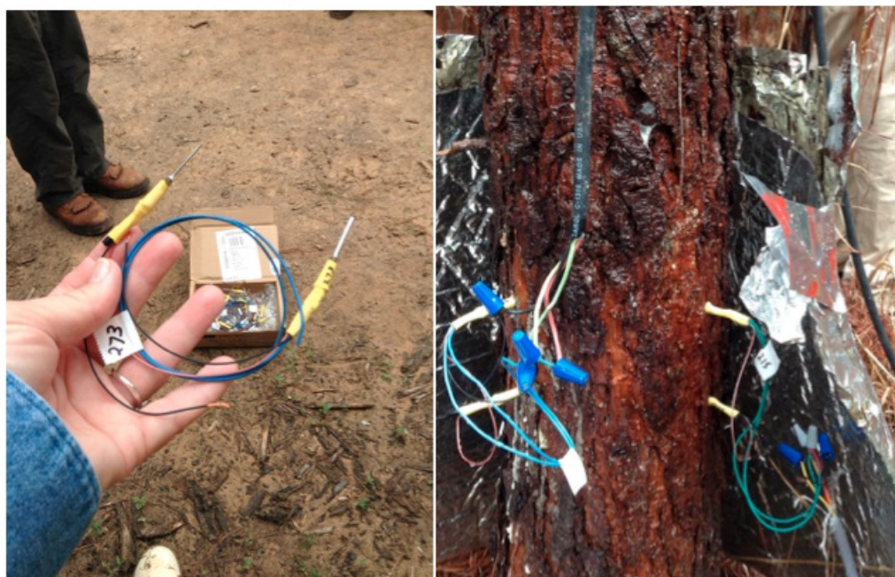
Sap Flux/Flow sensors used to measure sap flow and water usage in a tree
