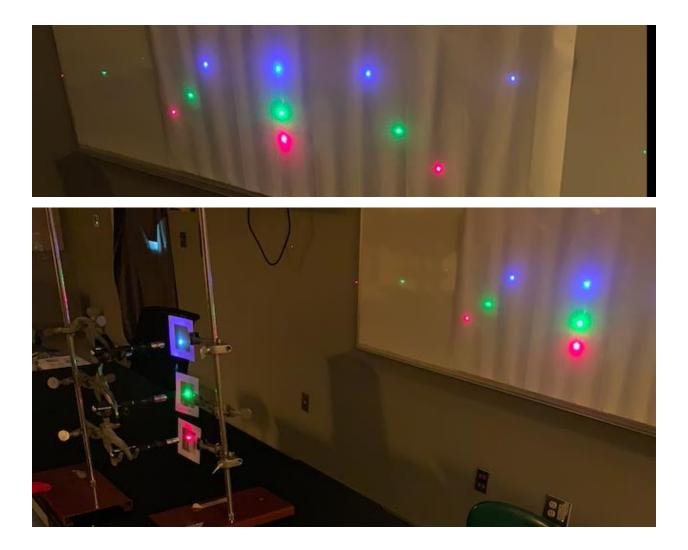
3) Shine the red laser through the diffraction grating with slits that are close together and with slits that are farther apart at the same distance from the screen. The top line is 500 lines/mm, and the bottom line is 1,000 lines/mm.
