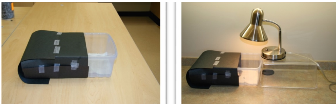
One chamber should be blocked from the light and the other side should allow for exposure to light.
