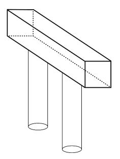
The design of the pier cap has the dimensions of  $5' \times 5' \times 20'$ . The design also requires a special emblem to be placed on the face of the pier cap.
