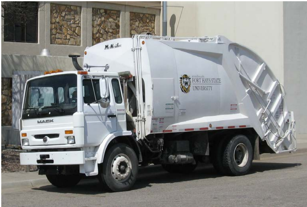
Mack MidLiner trash truck of Fort Hays State University.jpg. (n.d.). [Digital image]. Retrieved from https://commons.wikimedia.org/wiki/File:Mack_MidLiner_trash_truck_of_Fort_Hays_State_University.jpg
